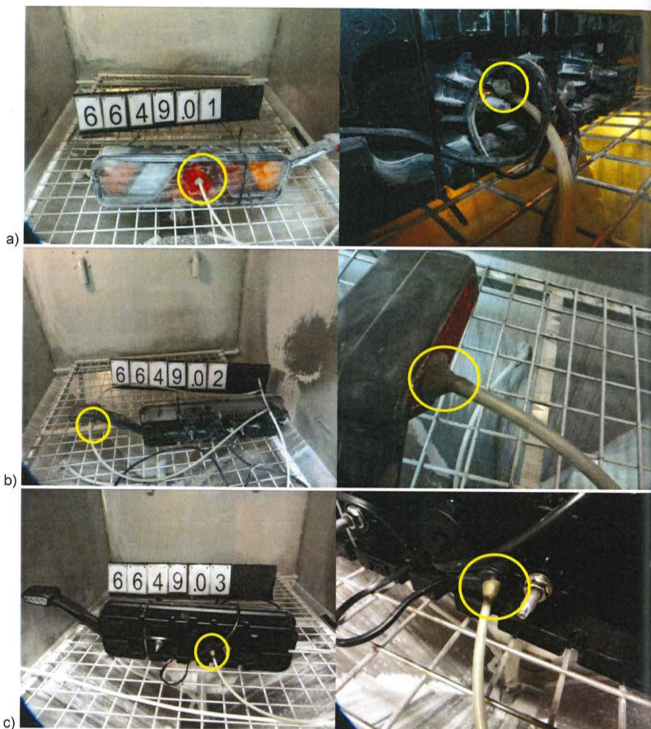
Photo. 6. EUT before IP6X test
