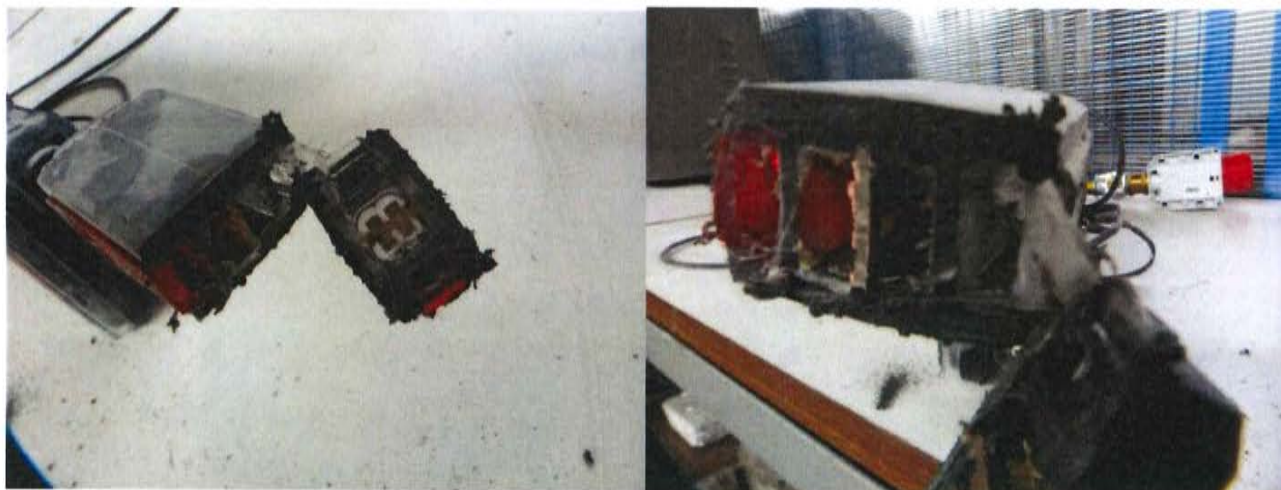
Photo. 9. Inspection of EUT 6649.02 after IP6X test
