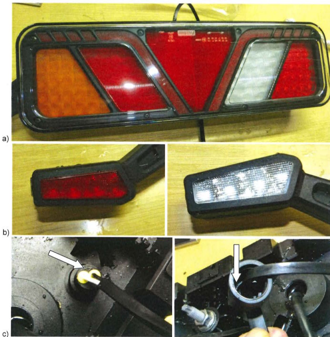
Photo. 4. Visual inspection after IPX8 test
